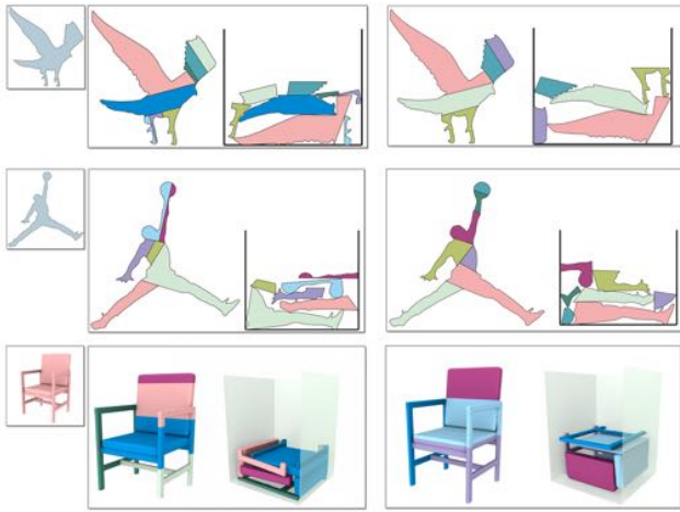
Figure 13: Contrasting DAP results without (left) vs. with (right) fabrication constraints. As opposed to optimization results without fabrication constraints, decrease in search time and increase in height of the final packing might occur, due to the more stringent search criteria enforced by the constraints. Note the elimination of small cuts (e.g., chair; eagle leg), small parts (eagle leg), and thin structures (many on Jordan, eagle, and top piece of chair).
