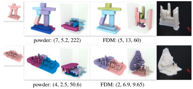
Figure 14: DAP results optimized for powder-based vs. FDM-based 3D printing. For each example, we show the input shape, the final (virtual) decompositions and packings with respect to the two optimization objectives, as well as a photograph of the FDM fabrication result. Part counts, heights(cm) and total volume( \text{cm}^3 ) of the vertical gaps are reported as well in vectors to show contrasts.
