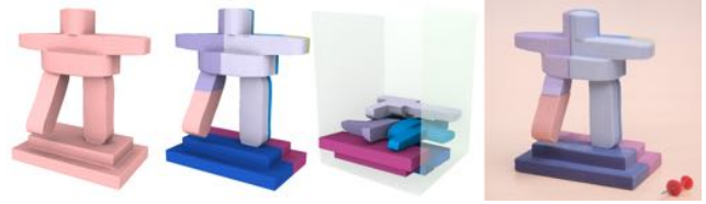
Figure 1: A 3D Inukshuk model (left) is decompose-and-packed (middle) for powder-based 3D printing. The fabricated pieces are assembled and glued together to form the final object (right).
