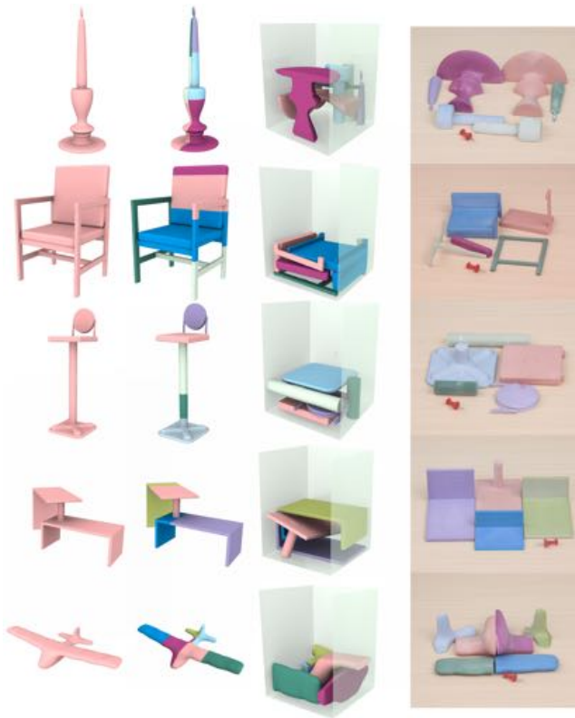
Figure 9: A gallery of 3D results from Dapper optimized for powder-based 3D printing (i.e., height minimization). For each example, we show (from left to right) the input shape, the final (virtual) decomposition and packing, and a photograph of the fabricated pieces. Part counts are shown in Table 1.
