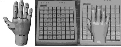
Fig. 4. Alphabetical code for the hand joints, left; specialized keyboard, center; position of hand over keyboard, right
