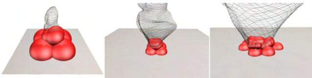
Figure 7: As the object gets closer to the plane the sphere hierarchies are refined (the camera is moved closer to demonstrate the sphere refinement)
